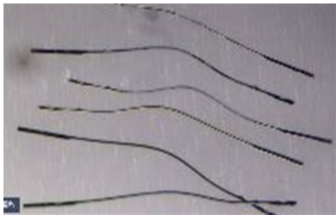
Deformed Probes due to current exceeding MAC
