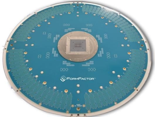
PCB and MLO design and manufacturing supports up to 1.6GHz and 3.2GHz
