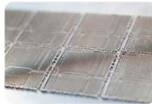
80um Pitch Grid-array MEMS Probe Head 30k pins, X8
